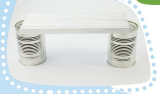
What can we change? Take another piece of paper and fold it like an accordion. Use this sheet of paper as a bridge and ideally place a simply folded piece of paper over the top so that you can place the weights on it more easily.
